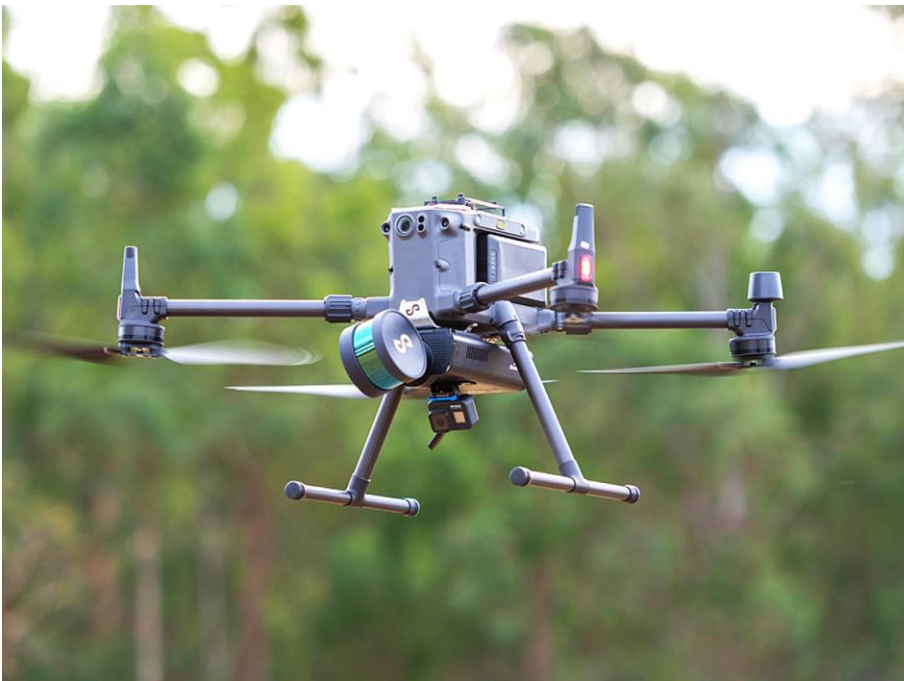
Figure 12: DJI Matrice M300 Drone with Hovermap LIDAR System and GoPro Colourisation
