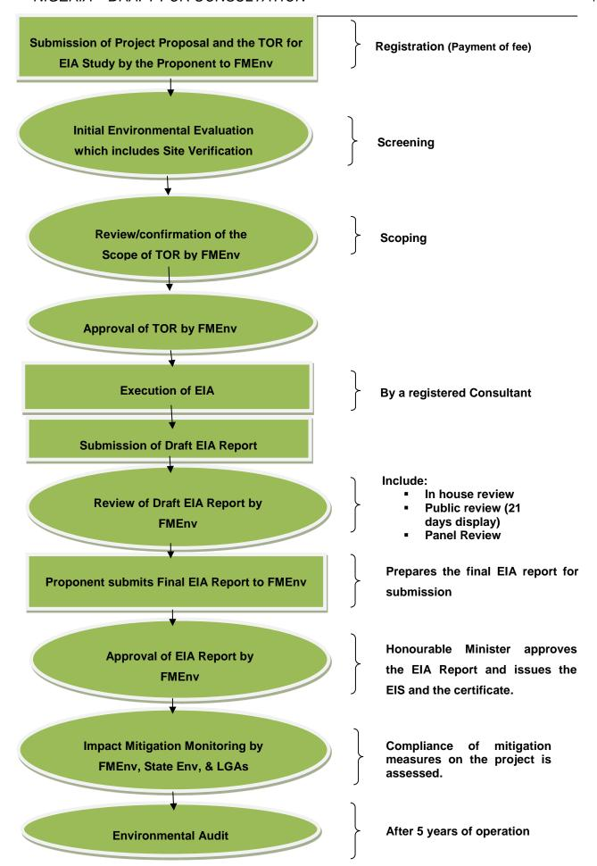
Figure 19.2: Flow diagram of the Nigeria EIA procedure
