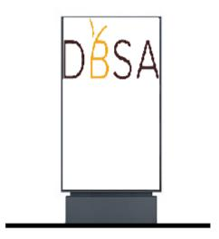
All LED signs should be connected to an existing 240V mains electrical system I, power will be sourced on nearby electrical pole or distribution network within the premises of DBSA. The LED signage electrical system should be designed to automatically switch ON at dusk by means of Photocell sensor.
