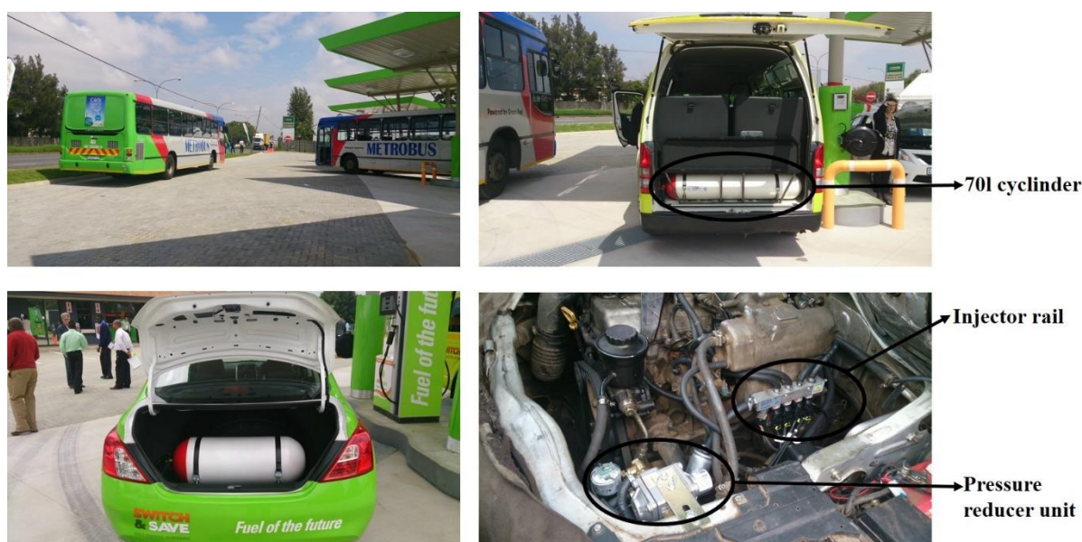
Figure 7-1 Metro buses, Mini bus taxis and saloon car fitted with natural fuelling system
