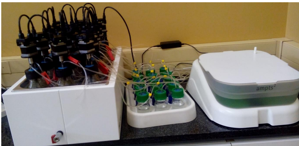
Figure 5-1 AMPTS II experimental setup for BMP analysis
