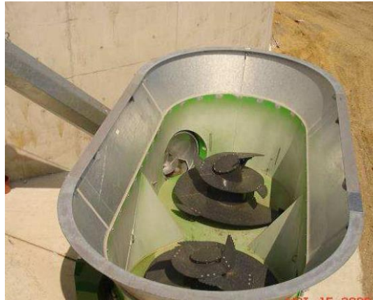
Figure 6-14 Feeding container equipped with screw conveyor, mixing and crushing tools
