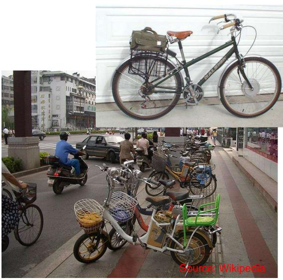
The e-bike can be effectively used for errands and trips where not much storage space is required, and is ideal for daily trips to work. The range of the bike is approximately 20km before the battery runs low and needs to be recharged. Pedalling is not required on the flat, downhill or gentle uphill (unless you wish to go faster), but is required to go up steeper hills comfortably.
