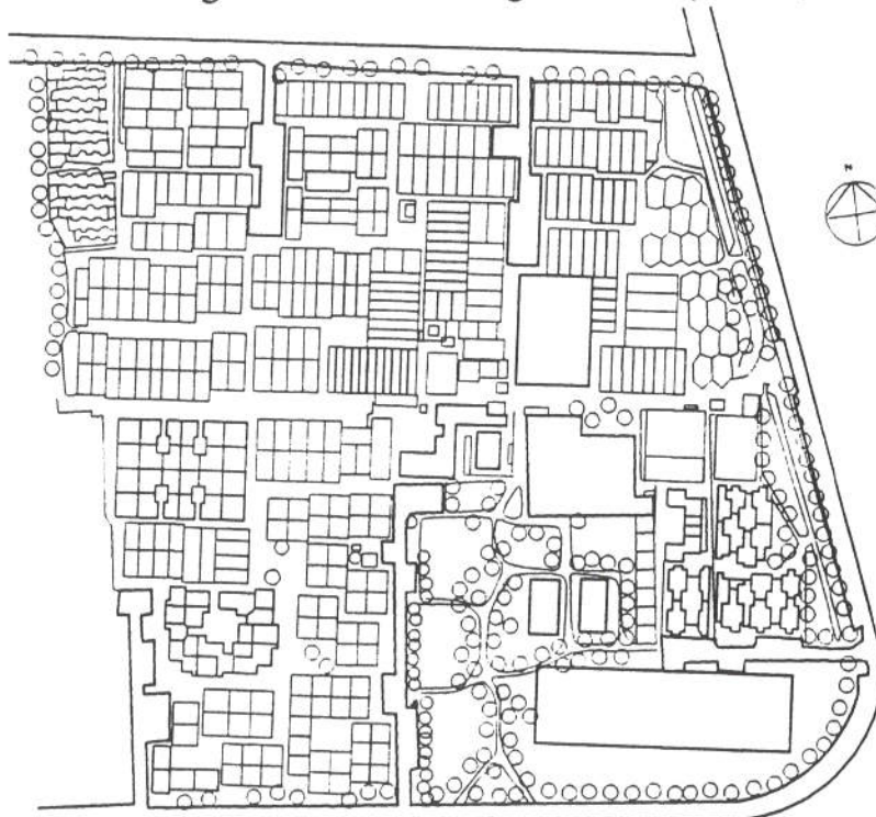
Figure 6. Experimental housing project, PREVI pilot project 1, Lima, Peru. Experimental area showing different plot shapes and groupings according to 23 selected design schemes. (Source: Fromm, 1985).
