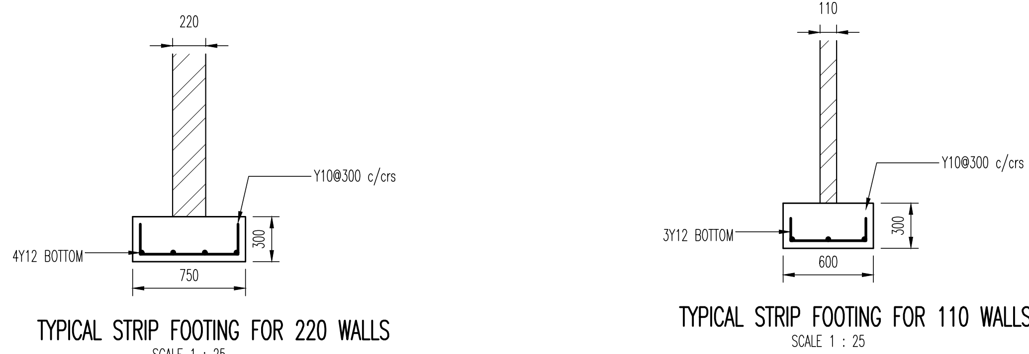
TYPICAL STRIP FOOTING FOR 220 WALLS SCALE 1 : 25
