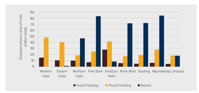
Figure 5.4: Expected hazard costs for the railway network
