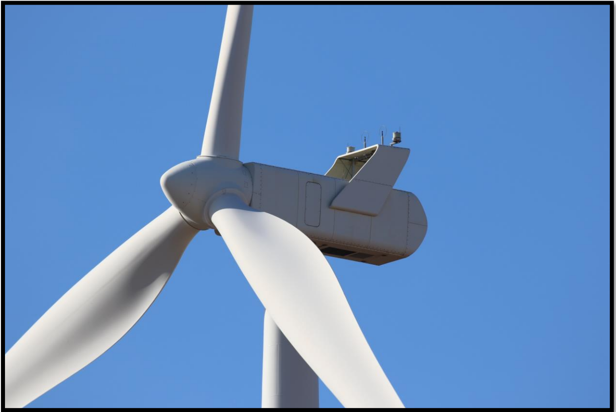
Photo 3.2: This photograph depicts a typical rotor with three blades attached to the hub of the wind turbine (Image courtesy of TMG).
